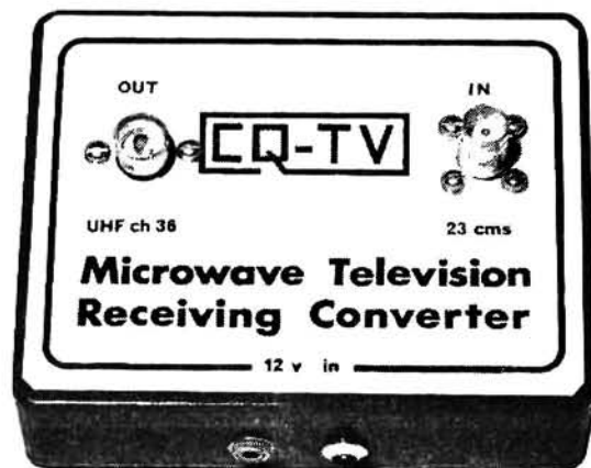
Probably the simplest of the commercial devices the CQ Centre receiving converter will allow initial ATV experiments to be made at 1.3GHz
